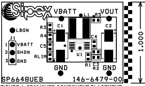
FIGURE 1: SP6648UEB COMPONENT PLACEMENT
