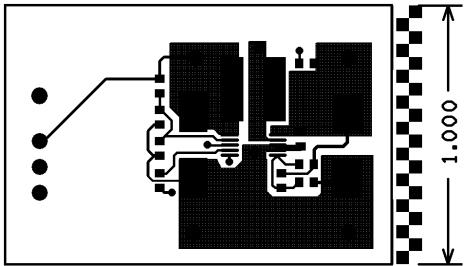
FIGURE 2: SP6648UEB PC LAYOUT TOP SIDE
