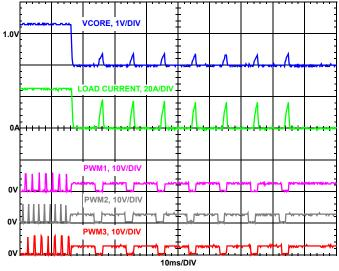
FIGURE 5. OVER-CURRENT PROTECTION
