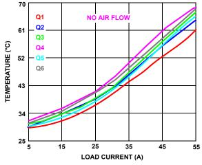
FIGURE 9. MOSFET TEMPERATURE vs LOAD CURRENT
