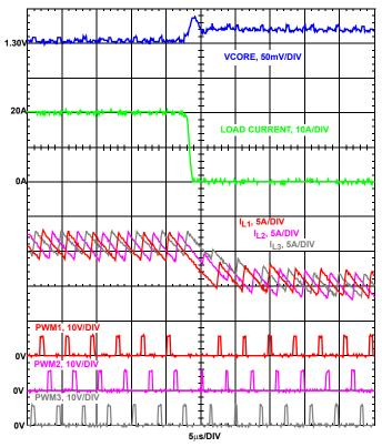
FIGURE 4. FALLING EDGE TRANSIENT RESPONSE
