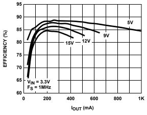
FIGURE 4. EFFICIENCY vs IOUT
