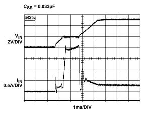
FIGURE 21. START-UP VOLTAGE AND CURRENT
