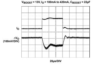
FIGURE 20. BOOST CONVERTER TRANSIENT RESPONSE
