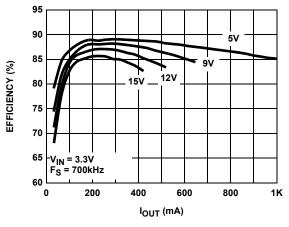
FIGURE 2. EFFICIENCY vs IOUT
