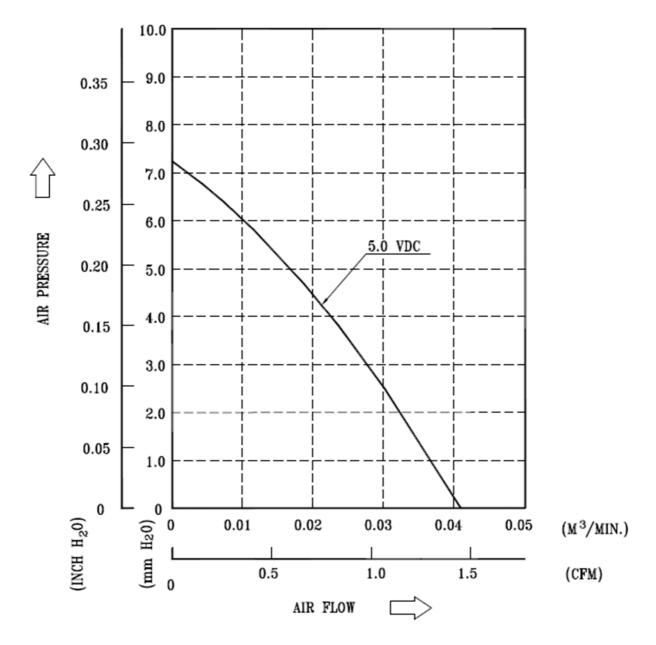
\*TEST CONDITION: INPUT VOLTAGE-----OPERATION VOLTAGE
