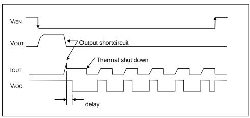
Figure 40. Over-current detection, thermal shutdown timing (BD82000FVJ)
