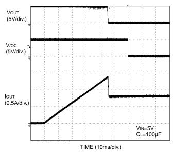
Figure 33. Over-current response ramped load
