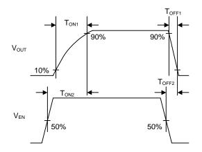
Figure 3. Timing diagram (BD82001FVJ)
