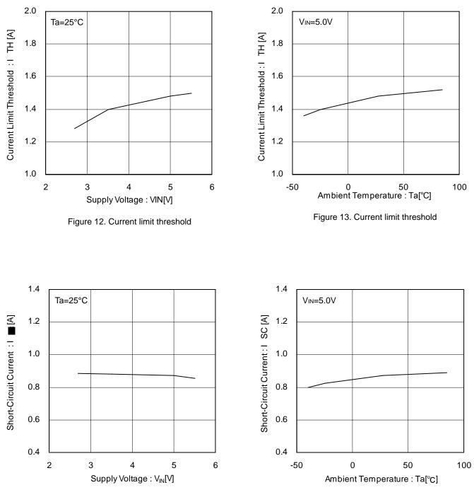
Figure 14. Short circuit current
