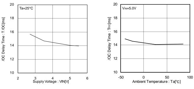
Figure 28. /OC delay time
