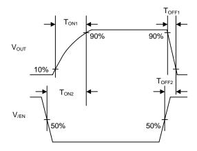
Figure 2. Timing diagram (BD82000FVJ)
