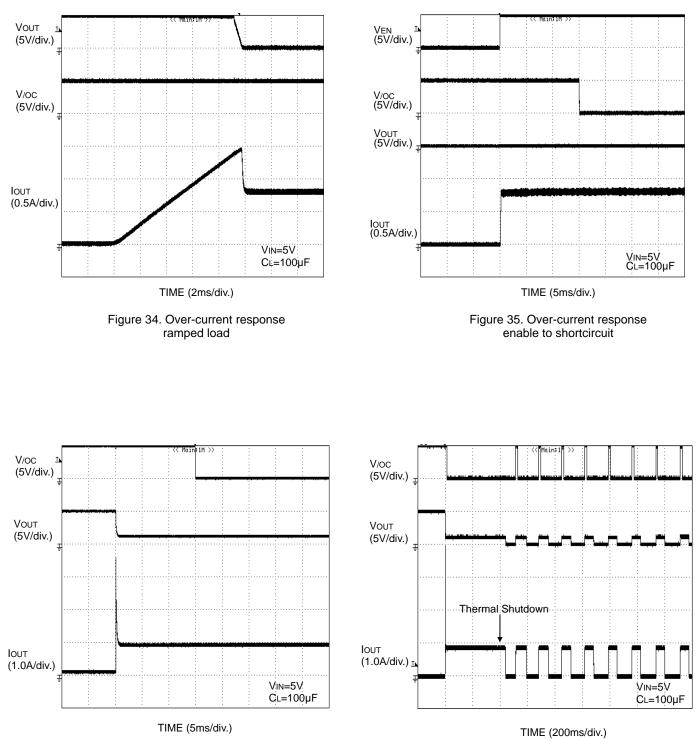
Figure 36. Over-current response  $1 \Omega$  load connected at enable
