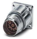
Device connector, front mounting, straight, SPEEDCON locking, M17, Number of positions: 8, Type of contact: Socket, Crimp connection, Axial O-ring, 4xØ2,7, shielded: yes, Flange dimensions: 21.6 mm x 21.6 mm
