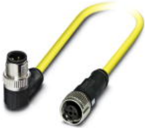
Sensor/Actuator cable, 4-position, TPE, yellow RAL 1021, Plug angled M12 SPEEDCON, A-coded, on Socket straight M12 SPEEDCON, A-coded, Cable length: 0.5 m
