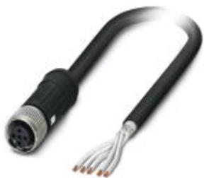
Sensor/Actuator cable, 5-position, PE-X halogen-free, black, shielded, free cable end, on Socket straight M12 SPEEDCON, A-coded, Cable length: 5 m, For railway applications
