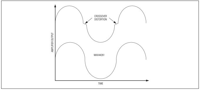
Figure 2. Crossover Distortion of Typical Amplifiers
