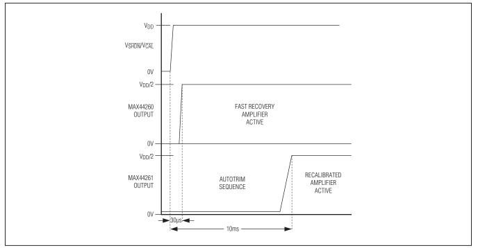
Figure 3. CAL vs. SHDN Input Operation
